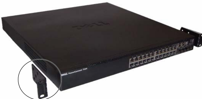
Figure 1-11. Fixation des supports
